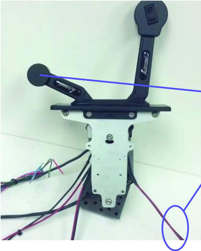
Shift lever in Forward position will close highlighted circuit.
